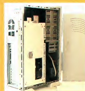
The EZPC Tower system showing the A1200, the PC rear sockets, card slots and removable side panels
